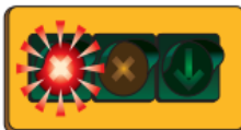
Control signal: Placed over lanes to indicate which ones are open for driving. Here: RED = do not drive in Right lane.
